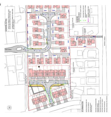
SmartMaps show Beverly Tce has an existing 650 Dia pipe network connected to Lincoln Rd which is 1050 Dia. The justification to bring these pipes ahead of existing flood locations needs review. Drawing is of the approved campsite development that disposes flood water onto roads not prepared for stormwater flow paths.
