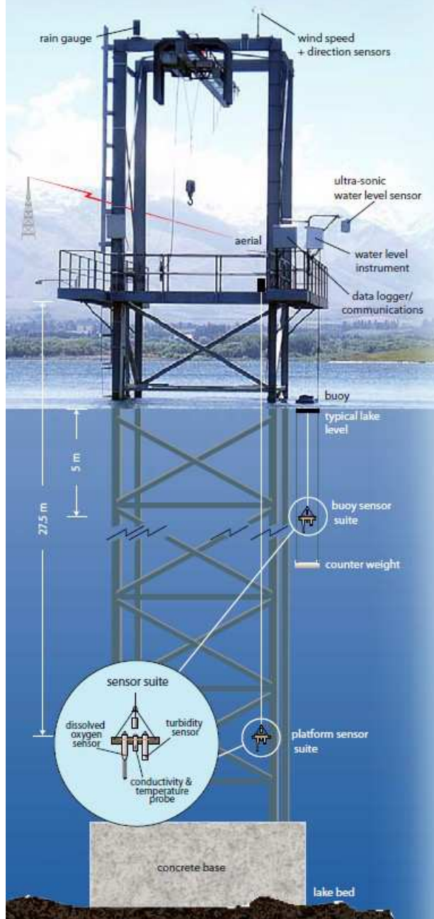
Figure 6-9: NIWA Instrument Services monitoring instruments attached to the offtake valve tower in Opuha Dam. For more information, contact NIWA Instrument Services (03) 348 8987. [With permission from NIWA].
