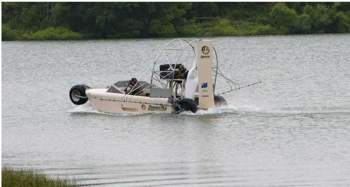
Figure 5-10: Spraying alum onto the surface of Lake Okaro. The air boat was fitted with GPS navigation to control where the spray was applied.
