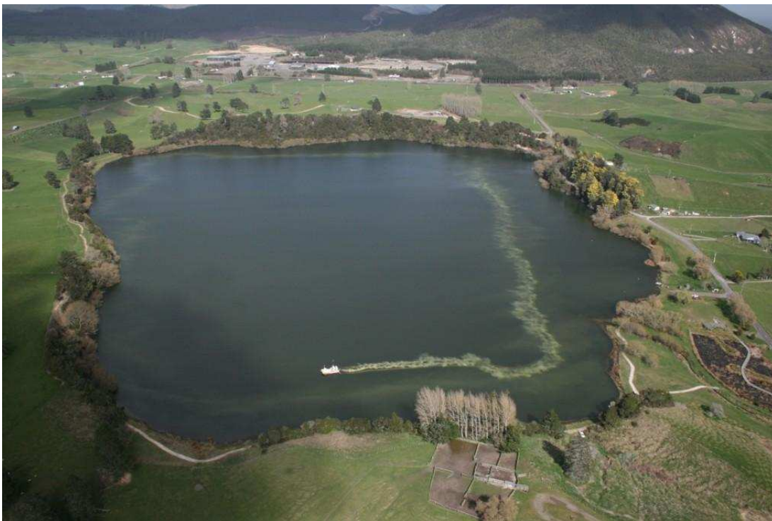
Figure 5-12: Application of Aqual P™ as a slurry from a barge on Lake Okaro. The barge position was controlled using GPS navigation. [Photo: Andy Bruere, Bay of Plenty Regional Council].
